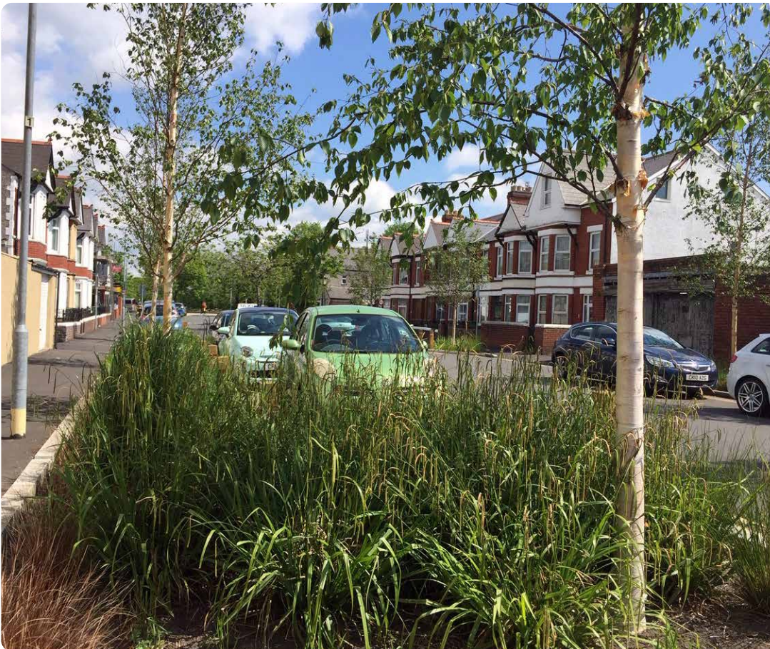
Figure 18: Example of a rain garden next to public highway
