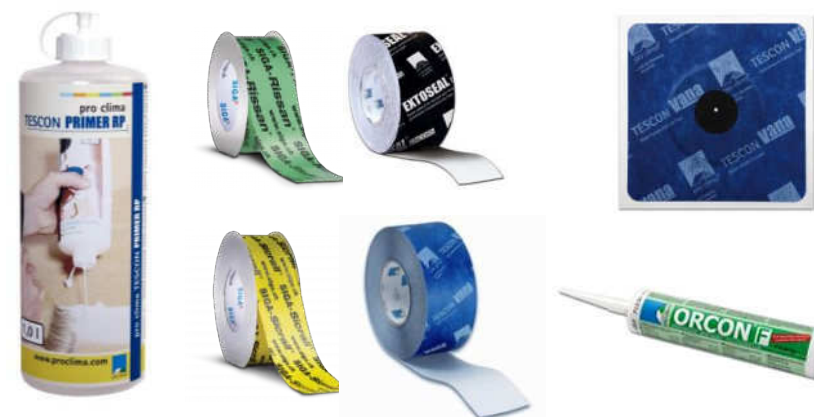
Components of the airtight layer are primarily connected together with tapes. Appropriate primers should be applied to certain surfaces before taping to ensure adhesion. Airtightness grommets and specialised long-life sealants are also available to assist with more specialist junctions in construction.
