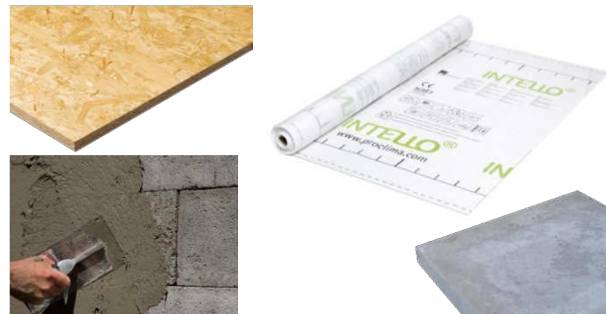
Large airtight surfaces within buildings are typically created from airtight OSB, parge coat and wet plaster applied over blockwork, concrete castings, or specialised airtight membranes. Do not use cheap polythene membranes, as these are fragile and lack the rigidity to tape without creases that cause leaks.
